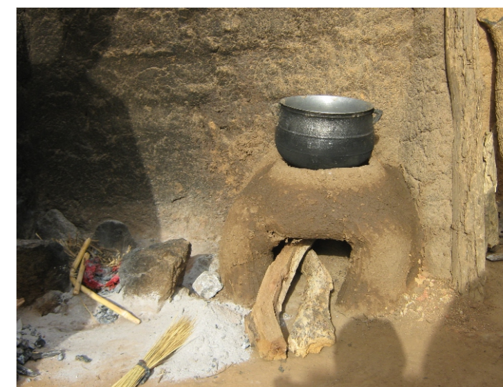
Fuel efficient wood stove made of locally available materials
